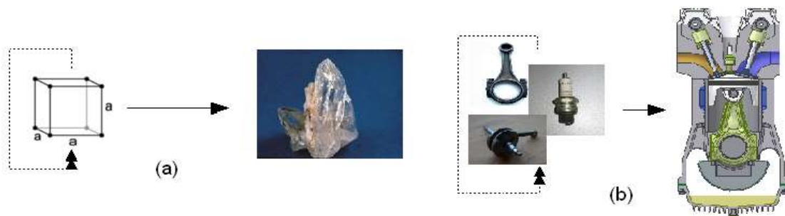
Fig. 3: In (a) the unit cell (in this case a cube as the most symmetrical structure of a crystal) recombines with identical structures via any of the 6 surfaces. In case of an engine (b) we add versatility to the system by having families of identical elements with different properties that may also exhibit a wider variety of interaction surfaces.
