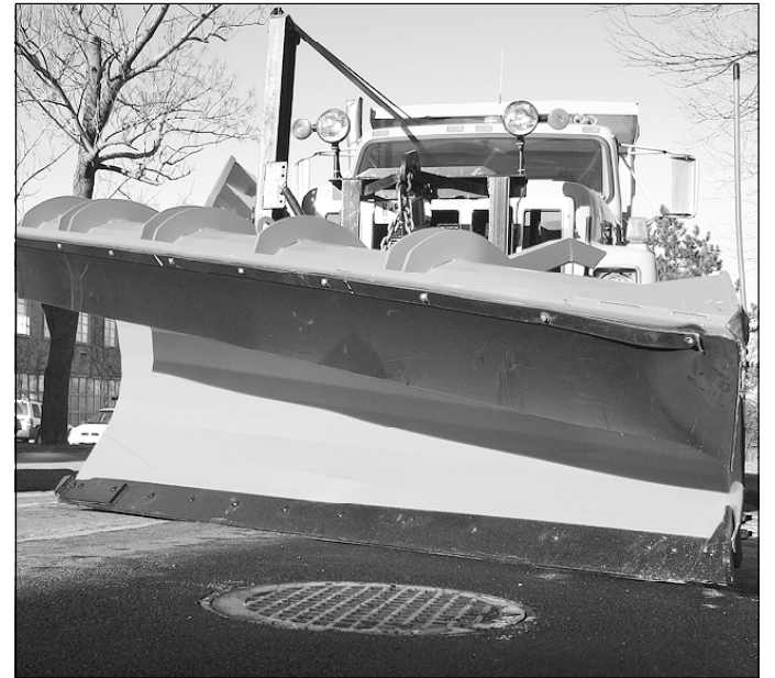
A recently patched manhole sits in front of the plow, a potential hazard for the workers if the patching deteriorates.
