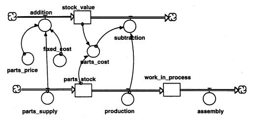
The instantaneous value of the parts\_stock is the integration of the input-stream added and the output-stream subtracted. Any material flow in the process-chain is in a similar way coupled to a flow of value (dynamic picture of the value added chain). For Activity-Based-Costing the process-chain-model with acounting attributes gives all the cause-effect information and insight to select the measures that really have impact.
