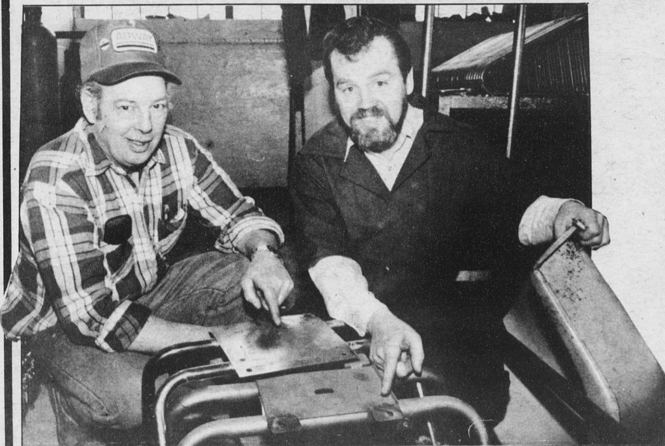
A $500 IDEA he had is pointed out by Woodward, left. He won the suggestion award for an idea for a replacement plate design. Rick Potter, who is also vice president of the CSEA Local at Great Meadow, shows the previous, easily broken, saddle strap plate design replaced by Woodward's invention. It will save the state thousands of dollars formerly spent repairing leg plates of metal chairs.
