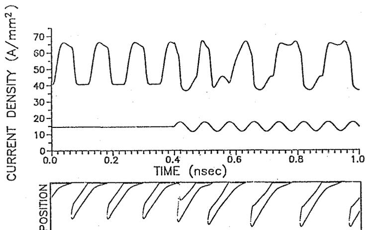
Figure 1. Onset of a 2:1 frequency-locked solution upon application of a microwave signal of amplitude  $A = 0.20$  and frequency  $f = 12.5$  GHz. By comparison with the undisturbed domain mode it is observed how the domains adjust their time of formation and their speed of propagation so as to entrain with the microwave signal. The upper panel shows the temporal variation of the current density and the applied field. The lower panel shows the propagation of domains through the crystal.
