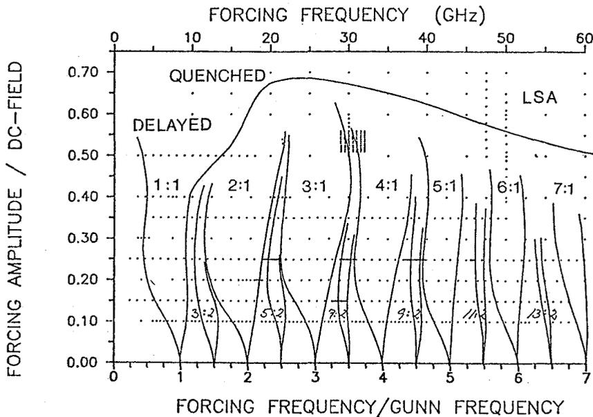
Figure 4. Phase diagram showing the distribution of behavioural forms as function of the frequency and amplitude of the applied microwave signal. Interspersed with the Arnold's tongues of frequency-locked behaviour one can find quasiperiodic solutions.
