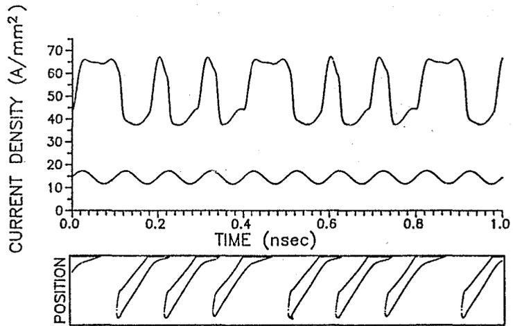
Figure 2. Stationary 4:3 frequency-locked solution obtained for  $A = 0.20$  and  $f = 10$  GHz. To keep in step with the microwave signal, the domain mode must delay the formation of every third domain.
