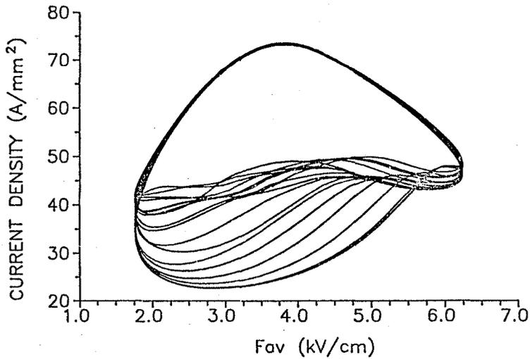
Figure 3. Phase-plot of the chaotic solution obtained for  $A = 0.56$  and  $f = 30.0$  GHz. In the neighbourhood of this solution we find a variety of complex solutions produced by period-doubling and mode-conversion of simpler frequency-locked solutions.
