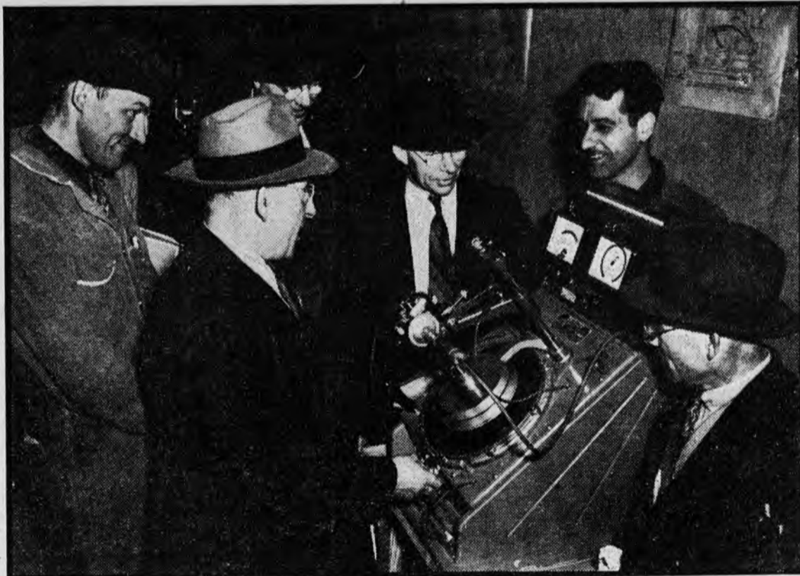
Here you see a group of New York City employees learning how to conserve automobiles in wartime. They're taking a course, and spend all day at it, in Central Motor Repair Shop, at 280 Avenue C, Manhattan. The gadget in this photo tests the distributor of an auto for cam angle and timing (if you take this course, you understand what that means). Idea is right in the title of the course: "Wartime Automotive Conservation and Maintenance."
