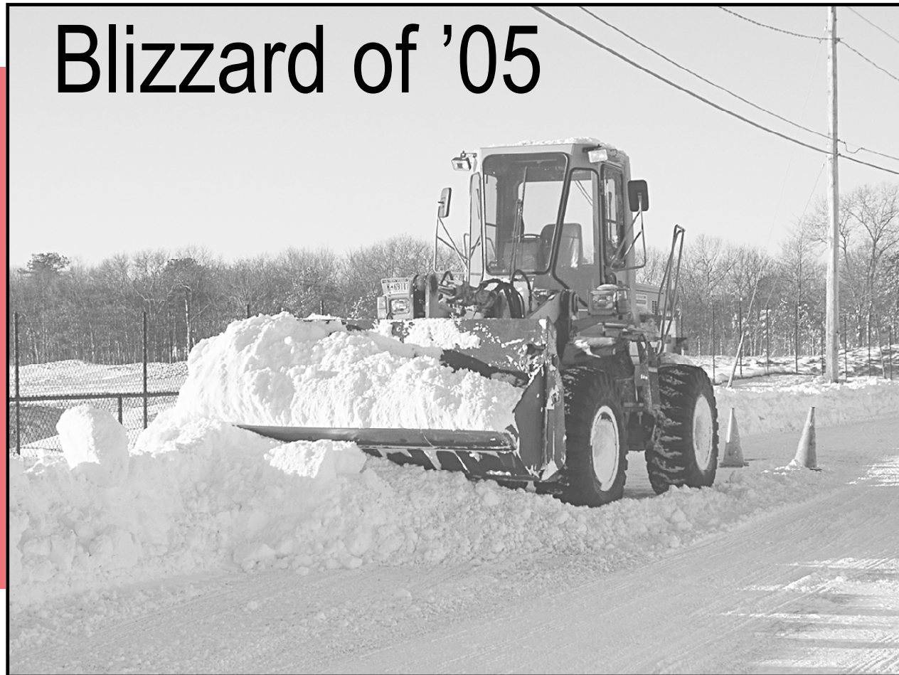
This payloader cleared heavy snow drifts from the road, but got stuck after diesel fuel froze because of the cold.
