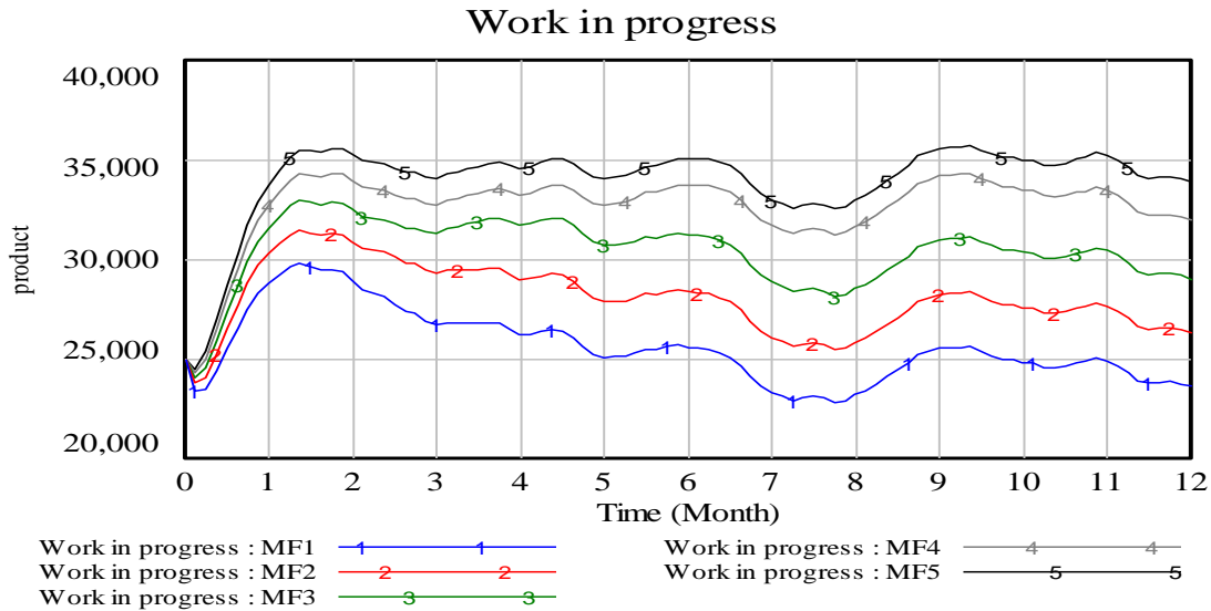
Figure 3: Behaviour of WIP for various machine failure rate.
