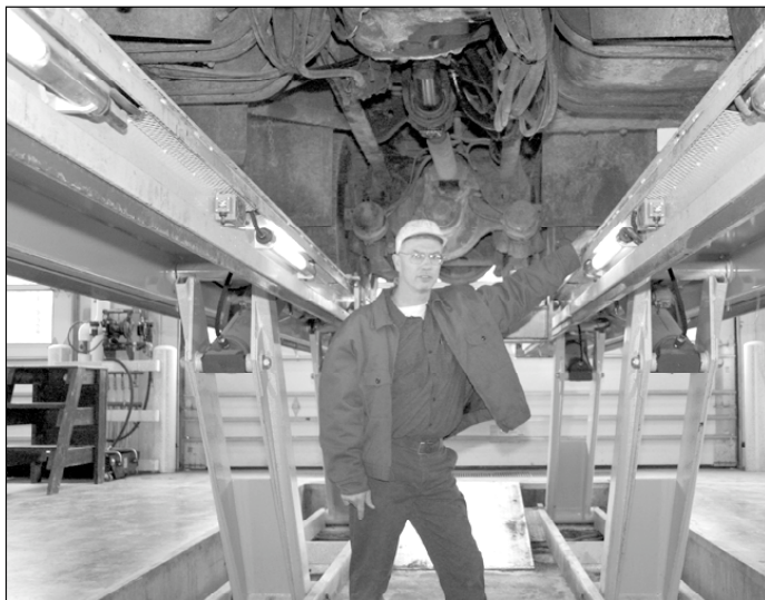
CSEA member and heavy equipment mechanic Paul Victory stands under a truck on a new hydraulic lift. The truck previously could have only been put on a ramp to repair.
