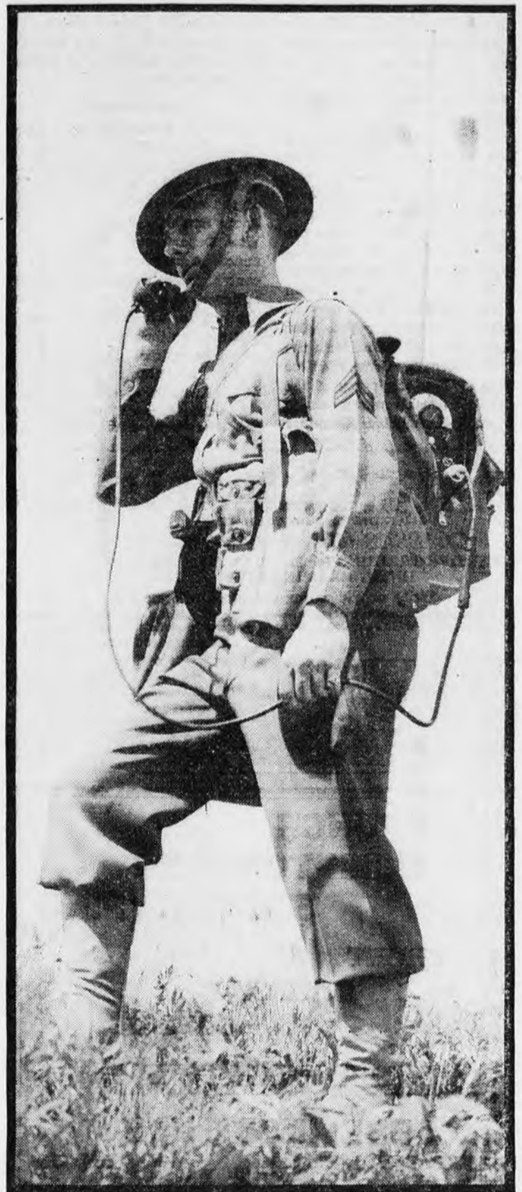
A U. S. Signal Corps soldier using the army two-way portable radio transceiver which provides communication with other men so equipped. Unobstructed, the range of this set will extend a considerable distance. It weighs about half as much as the regular infantry set . . . Radio work is one of the very best studies a man can undertake these days, if he's looking to get places.
