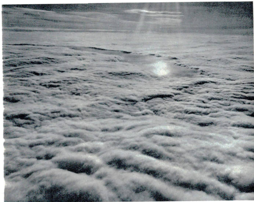
Fig. 15. Portion of 15 miles long "L" pattern produced with about 1-½ pounds per mile of dry ice which resulted in overseeding effect. Note reflection. Flight 3, April 7, 1947, Project Cirrus . (Official Photo, Signal Corps Engineering Laboratory.)
