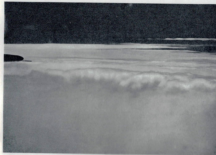
Fig. 24. Large area of supercooled stratus cloud modified with dry ice. Flight 83, Project Cirrus . (Official Photo, Signal Corps Engineering Laboratory.)
