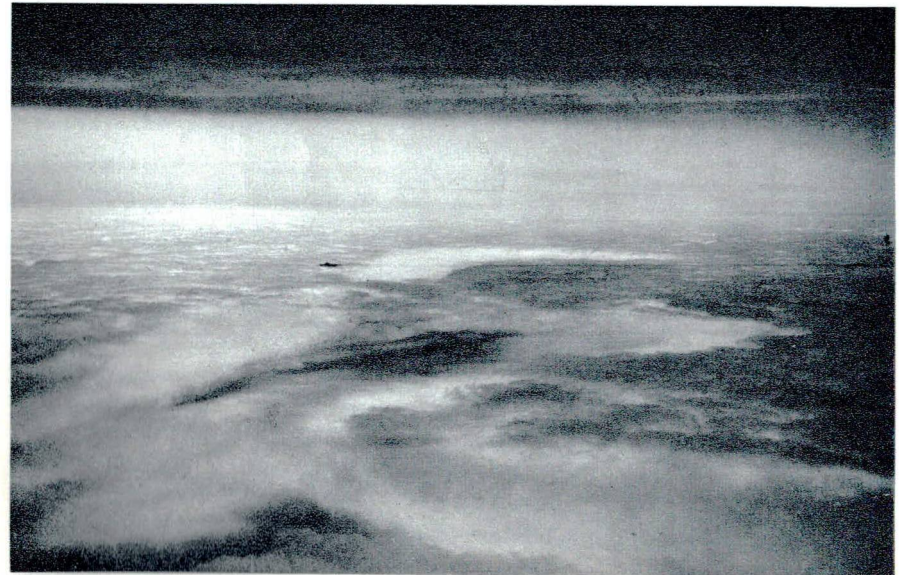
Fig. 20. View of two "L" type patterns produced by dry ice seeding of supercooled stratus cloud. Flight 80, March 31, 1949, Project Cirrus . (Official Photo, Signal Corps Engineering Laboratory.)
