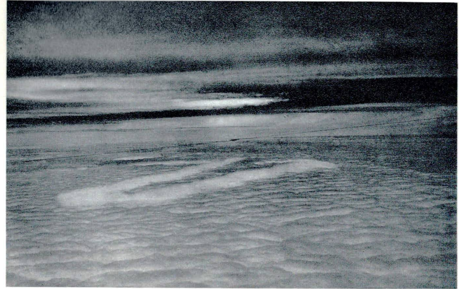
Fig. 19. View of "Figure Four" pattern produced by dry ice seeding. Legs 10 miles long. Flight 73, March 10, 1949, Project Cirrus . (Official Photo, Signal Corps Engineering Laboratory.)
