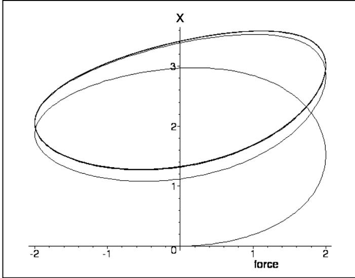
**Fig. 6:** Dynamic hysteresis curve with  $F_0=2$ ,  $T=4$ ,  $\tau=1$  showing oscillation around the equilibrium point at  $x=+2.828$ . The trajectory circles around the positive equilibrium of the potential  $V(x)$ , because it started at  $x=0$  with the force increasing from zero to positive values.
