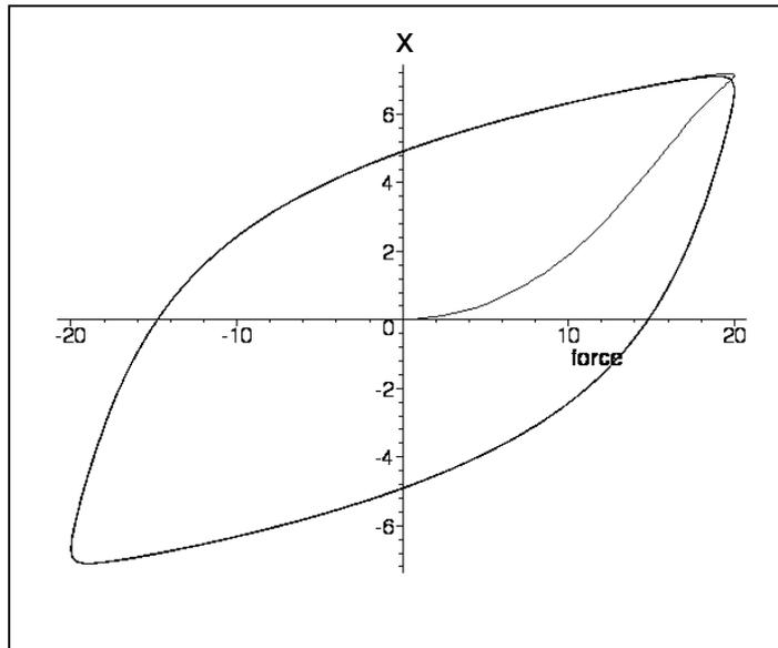
**Fig. 7:** Repetition of the simulation shown in Fig. 6 but with the force increased tenfold ( $F_0=20$ ,  $T=4$ ,  $\tau=1$ ). The resulting dynamical hysteresis curve is different from the quasi-stationary curve shown in Fig. 5, because the system follows the variation of the external force  $F(t)$  with a non negligible delay resulting from its internal time constant  $\tau=1$  being in the same order of magnitude as the period of the external force  $T=4$ .
