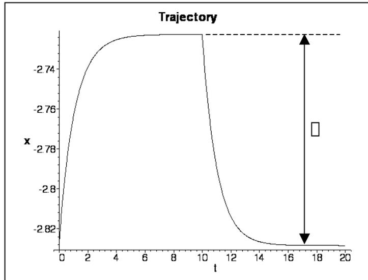
**Fig. 8:** Trajectory beginning at the left equilibrium ( $x_s = -2.828$ ) for a constant external force  $F_0 = 0.1$  in the time interval  $t = 0 \dots 10$ . For  $t > 10$   $F_0 = 0$ . A new equilibrium position is found after a few  $\Delta$  ( $\Delta = 1$ ) with a distance  $\Delta$  from the stable force-free equilibrium point of approximately  $F_0 \cdot \Delta = 0.1$ . The simulated distance between the two equilibria is about 0.105 as indicated by the double arrow.
