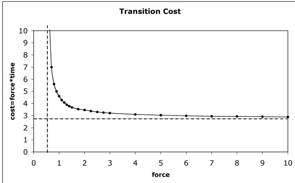
**Fig. 9:** Transition cost ( $F_0 \cdot T$ ) versus force ( $F_0$ ) for  $\beta = \alpha = 1$  necessary to bring the system to the critical point  $x=0$ . The broken vertical line shows the first and the broken horizontal line the second condition of (17). To induce a state transition, a minimum force of about 0.5 is needed; the lowest transition cost of nearly 3 is approximated when large forces are applied.
