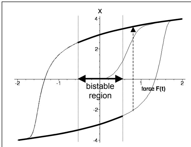
**Fig. 5:** Quasi-stationary hysteresis curve for the potential given in Fig. 4 with  $T=60 \gg \tau=1$ . The simulation started at  $(0/0)$ , giving an aperiodic initial trajectory, before the system response is periodic. Note the ordinate intersection points  $(0/\pm 2.828)$  showing that the system is able to follow the variation of the external force  $F(t)$ . Only the bold portions of the hysteresis curve are quasi-
