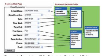
Figure 1. Shredding XML Data into Relational Tables.
