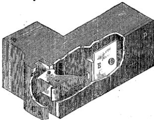
Mr. Ham thus describes his lock: "It is a spring lock for cell doors, which contains the elements of strength, simplicity and security in an eminent degree, as it fastens by merely shutting the door (requiring a key only to open it), and when fastened, the door is held as in the grasp of a hand, a
