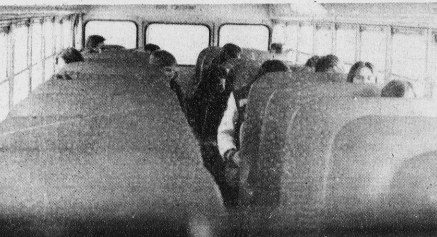
DIFFERENCE IS CLEARLY EVIDENT between higher backed seats and lower backed seats in these two photos taken from a school bus driver's seat and through the driver's rear view mirror. In the newer, 28-inch high seats, left, these high school students are barely visible in the
