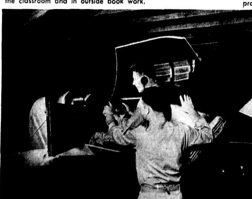
In the little plane that never leaves the ground, Cadet Harris receives training in blind flying. The Link Trainer is the bane of many cadet's existence, but not for Harris who can fly like a bat at night.
