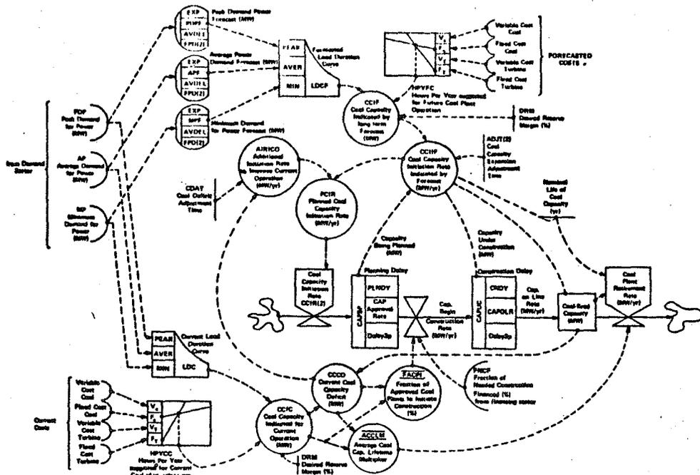
Fig. 2. Modified DYNAMO flow diagram showing coal capacity initiation rate.
