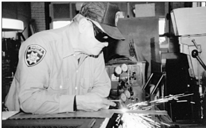
Maintenance Mechanic Ed Melin builds and repairs the gates, grates and any other metal security fixtures used at the jail. Above, Melin is cutting with a torch.
