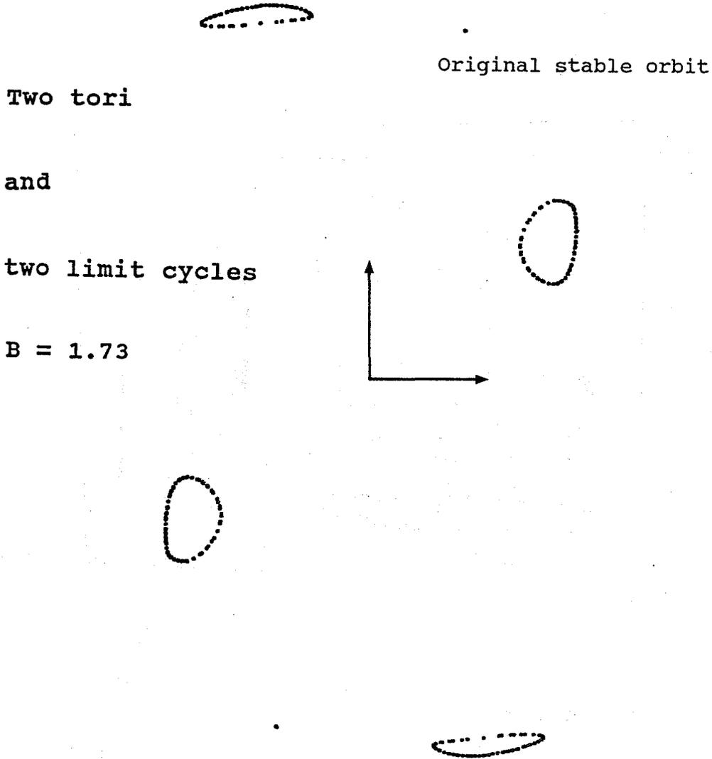
A two-dimensional projection of the Poincaré section for  $B = 1.73$ . The two symmetric period-1 orbits remain stable, while the two symmetric period-2 limit cycles each undergo a torus-bifurcation when  $B$  is reduced below 1.75. This means that the trajectories are located on the surface of a torus (or a doughnut). In this case the oscillations never repeat themselves. The solution is said to be quasi-periodic.
