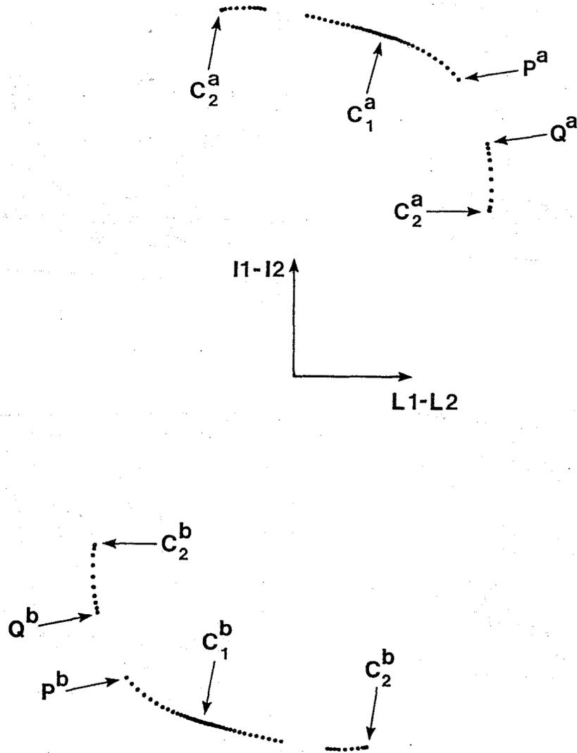
A two-dimensional projection of the Poincaré sections for  $B = 1.8$  reveals four co-existing attractors. The three-dimensional cutting-plane passes through the unstable equilibrium point ( $L_1 = L_2 = L_3 = I_1 = I_2 = I_3$ ) with a normal vector of  $(1,1,1,1)$ . Transient approaches to the four attractors are seen beginning at  $P_a$ ,  $P_b$ ,  $Q_a$  and  $Q_b$ , respectively. The corresponding stable solutions are denoted  $C_1^a$ ,  $C_1^b$ ,  $C_2^a$  and  $C_2^b$ .
