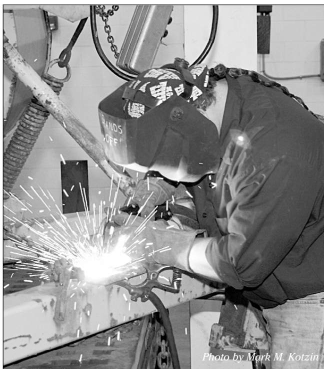
CSEA Onondaga County Department of Transportation member Brad Allen welds a repair to a snowplow blade, which took more than its fair share of abuse this winter.
