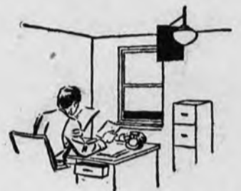
The same precautions are applicable to offices, stores, and all other commercial and industrial establishments. Office ceiling fixtures that are close to the window should be shaded on the window side as shown. When a store entrance is left open, all light sources visible from the outside must be covered on the side facing the open door.
