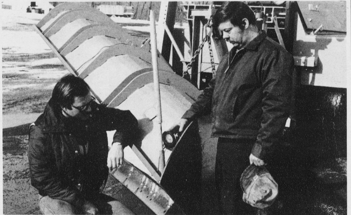
SAFETY WHERE IT COUNTS is demonstrated by Head Mechanic Ron Lawson, right, as Allen Rotach, president of CSEA Local 519 NYSDOT looks on. Lawson is credited with developing "Rudolph," a blinking light device for the tip of snowplow blades. Rotach and other plow drivers say the safety innovation has proven itself in snow conditions, both in driving and as a warning to oncoming motorists.
