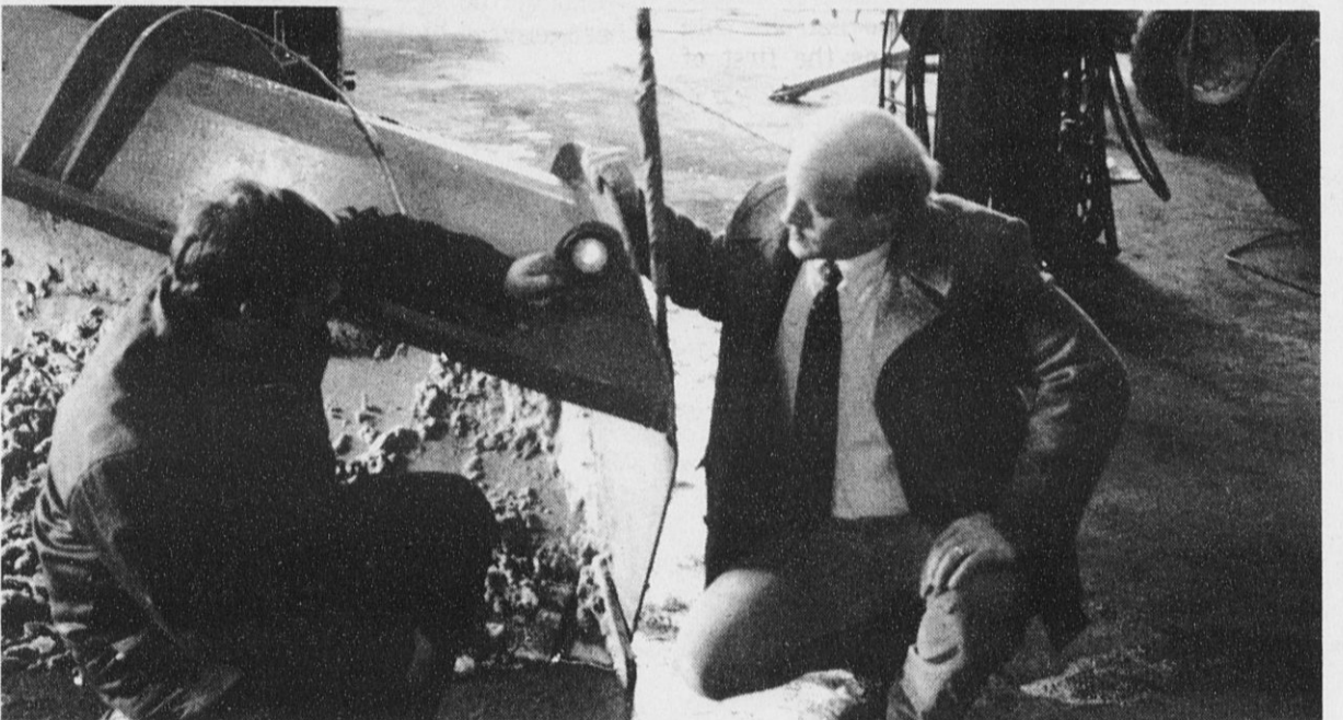
TAKING A CLOSER LOOK at 'Rudolph' in action is Chris Jamison, right, Region V OSH representative, as head mechanic Ron Lawson describes how the snowplow safety light works. The inexpensive safety device has been installed on all snowplows in the NYSDOT Wayne County residency and is credited with reducing plow/car incidents to zero in the past several years.
