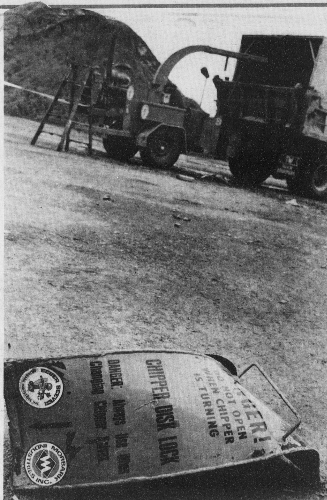
METAL COVER in the foreground was hurled against Richard Conrad, killing him, and landed more than 25 feet from the brush chipper in the background.
