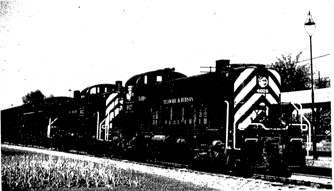
Alco RS2 #4025 leads the Laurentian at Montreal West on May 22, 1955. Note the spilled fuel oil under the “2” below the cab. The filler is one of the spotting features of the RS2, even after the D&H upgraded the units to RS3’s. Photographer is Skipper Clark; donated by Al Jacobsen. BLHS Collection.
