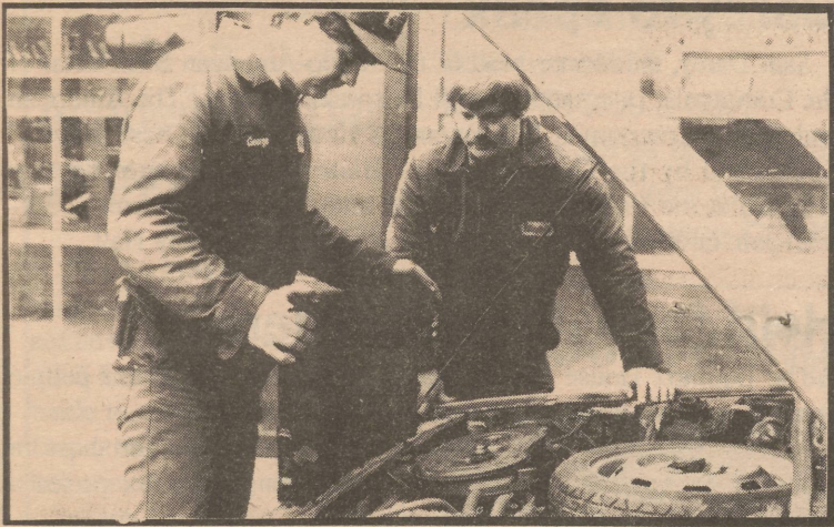
Staff Photo by Leanne B. Warshauer George Dunbrook and Ed Austro change a worn-out radiator, a common source of trouble in the winter.
