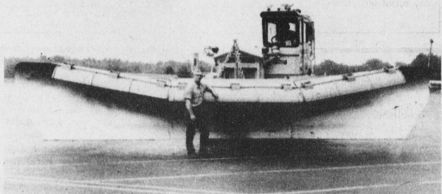
JOHN MacLEAN stands in front of a 28-foot snow plow which is used to keep the runway at Tompkins County Airport open during the harsh central New York winters.
