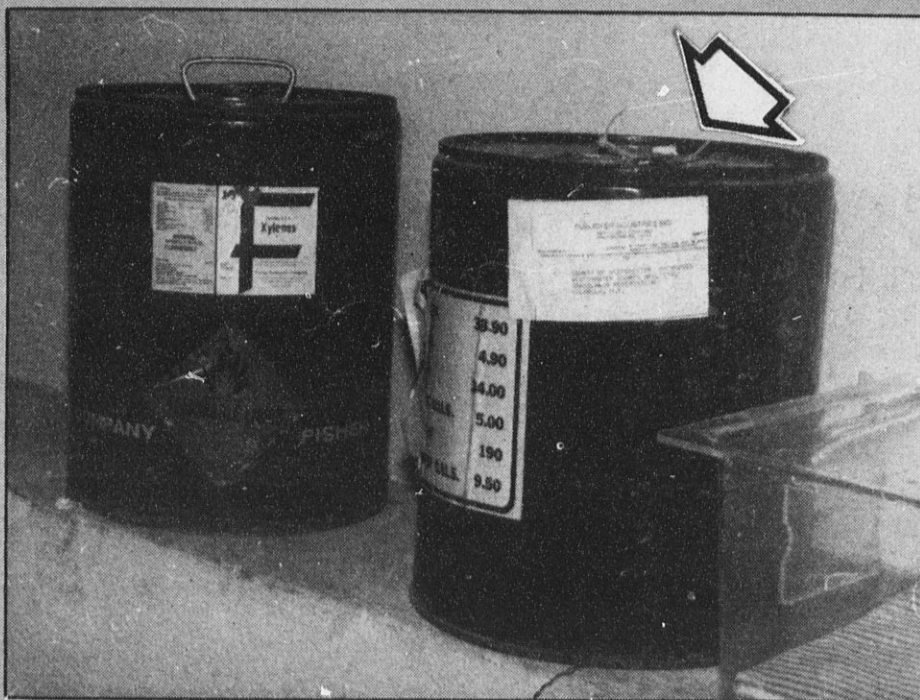
A CIGARETTE BUTT found on the top of this container was cause for alarm. The container still had a flammable chemical inside and was stored in a hallway where worker traffic is heavy.
